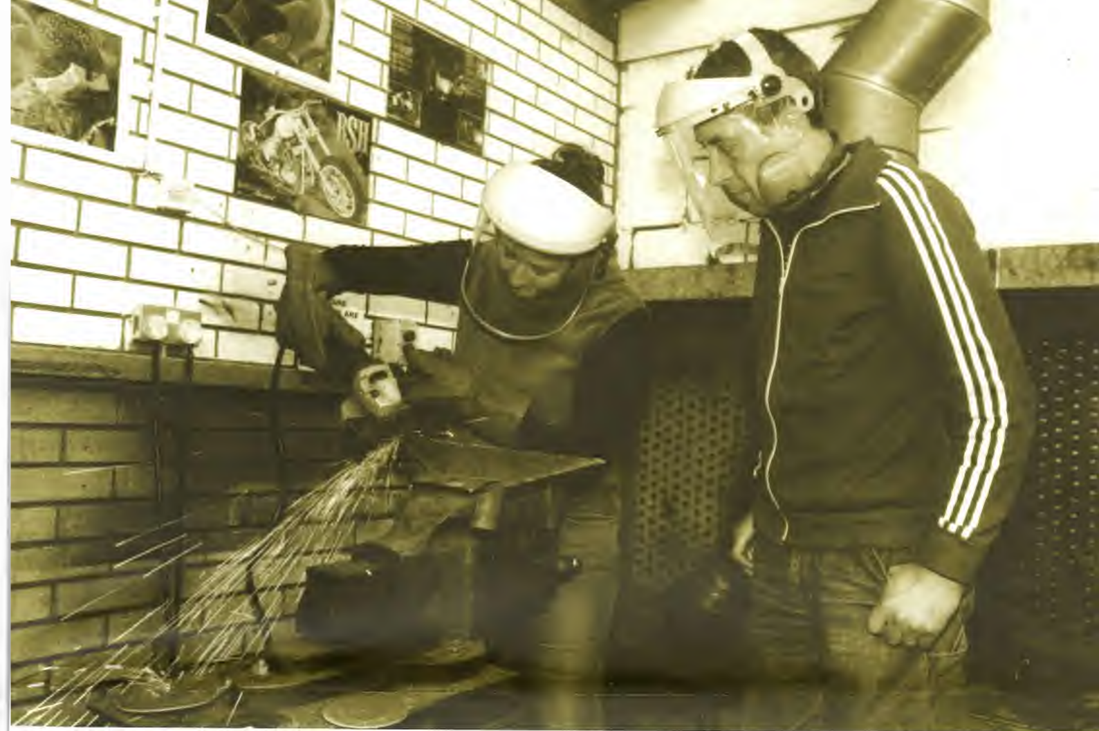
ABOVE: Warren Best, Technician Instructor in 3D workshop teaching angle grinding.
